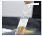
To avoid fluid leakage, squeeze the fluid from the top of the pouch downward into the bottom chamber. Tear off the plastic top above the white closure.
