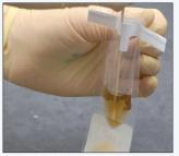
To admit the swab, open the pouch by pulling the closure tape middle tabs apart. Carefully squeeze a small amount of liquid back into the top chamber and knead the swab between the pouch walls. Remove swab and discard.
